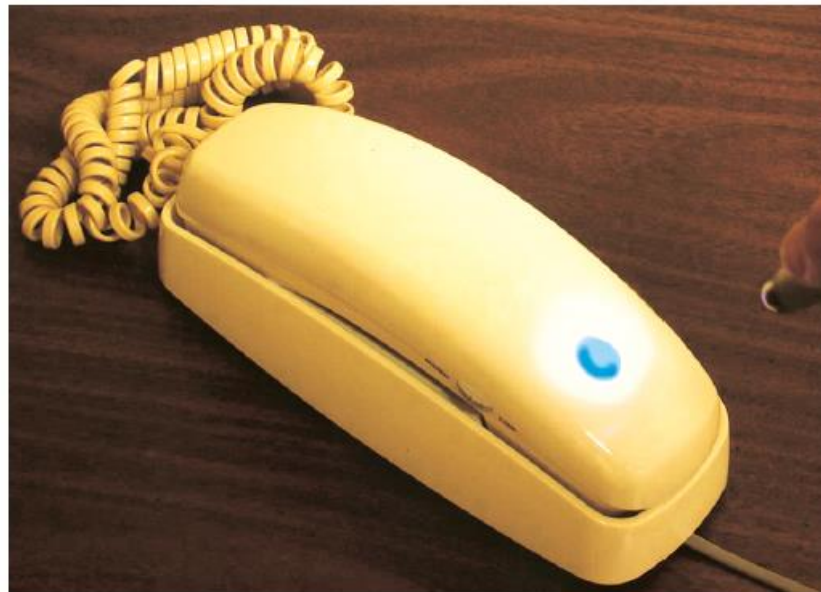
Figure 1. The manner in which a target is made visible on a bedside telephone, using a portable black light
